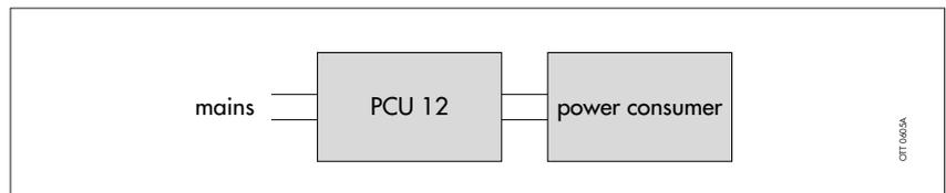
The power consumer is connected to the plug-in screw terminal strip on the PCU 12:
