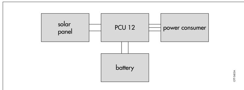
The solar panel current must not exceed 12 A, while the open-circuit voltage must not exceed 23 V (12 V in the case of nominal voltage). If the load current is greater than the solar panel current, the battery is discharged. When dimensioning the battery and the solar panel, you must ensure that the discharging of the battery is compensated for by a suitable charging cycle. The battery capacity must not exceed 200 Ah.
