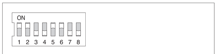
Fig. 20: Factory setting of the operating parameters.
